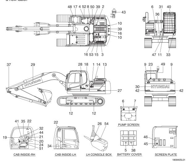
Air cleaner filter 19 Control ideogram 38 Electric welding 39 Turbocharger cover 20 Ref operator's manual **Falling** Radiator cap 21 Hammer 40 FOPS FOG plate **Fueling** 22 Safety front window 41 Caution (water separator, 23 Battery accident Safety rear window turbocharger)
